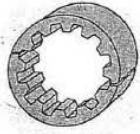
(E) shell of the internally toothed member ruptures
