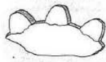
(C) teeth break at roots in a cantilever type failure similar to that of gear teeth
